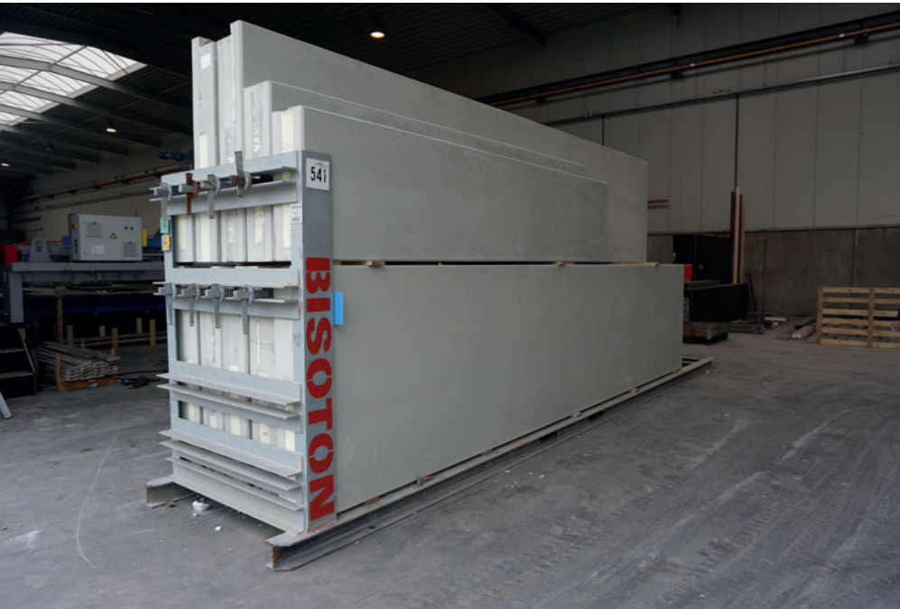
Finished sandwich elements made with the BT shuttering carrier system.
