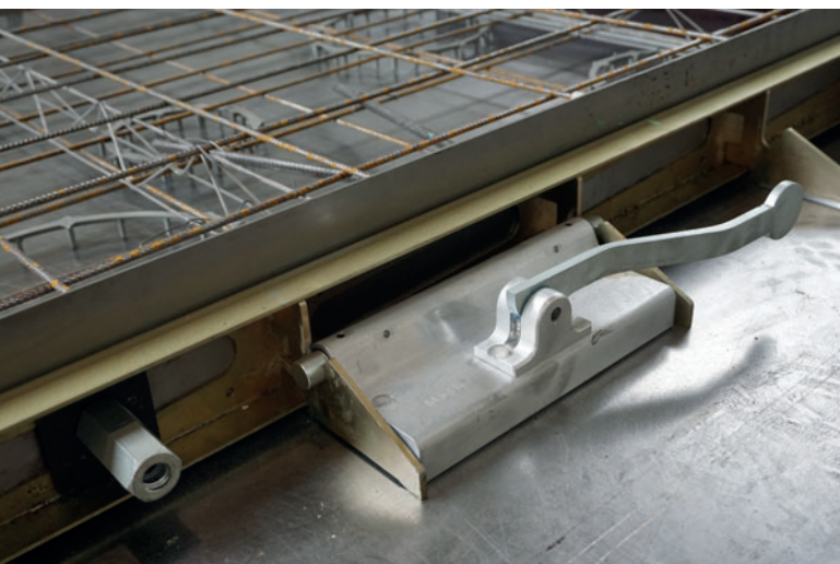
UniForm bolted shuttering sheet on MultiForm shuttering carrier: The shuttering was fixed with MagFly AP magnets.
