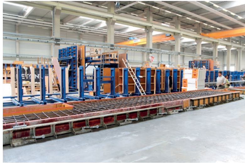
Overall view of finished formwork before concreting
