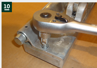
10: Firmly tighten the fixing screw
