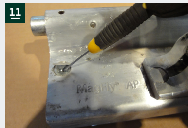
11: Reapply the cover cap by using silicone
