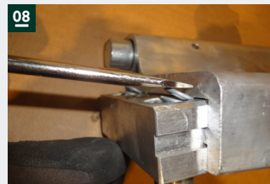
08: Carefully compress the springs and push them into the block
