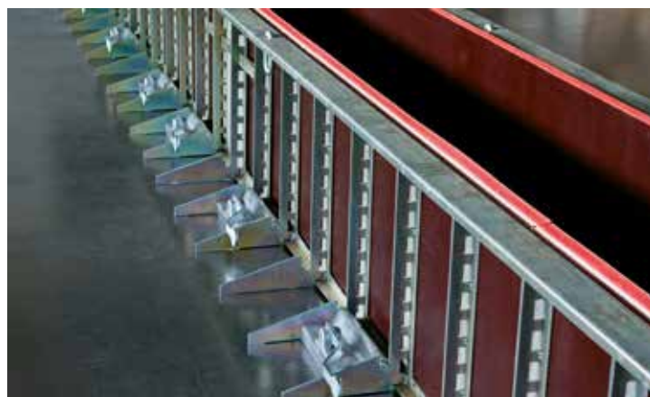
MultiForm shuttering system and MagFly AP as substitute for resource-intensive disposable wood shuttering
