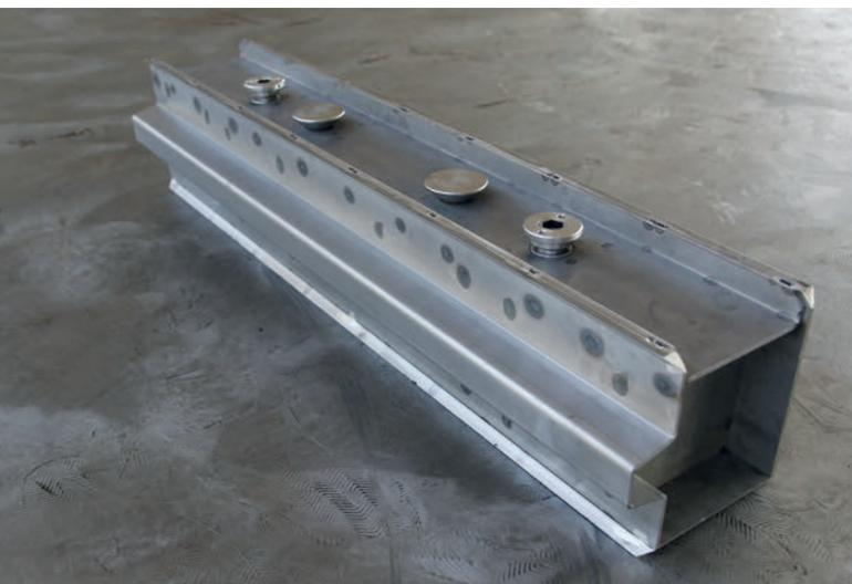
Special solid formwork with integrated magnets and holder for robot gripper
