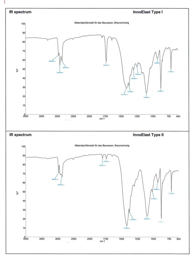
The infrared spectra were recorded in a wave number range between 4,000 cm<sup>-1</sup> and 600 cm<sup>-1</sup>. The coating thicknesses were selected to comply with the requirements of DIN 51451 in relation to the extinction ratios.
