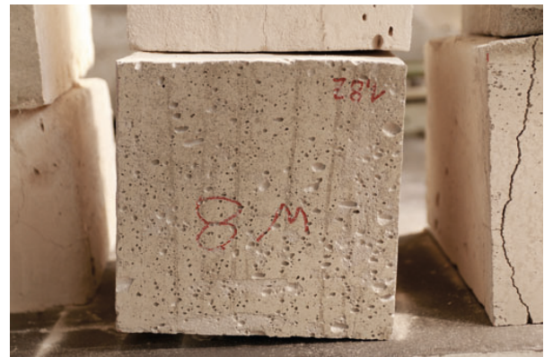
Fig. 2: Left: Five test cubes were cut out of the foam concrete wall at the bottom, middle and top to determine the density. The position of the cubes corresponds to the distance from the lower edge of the cut cube to the lower edge of the cast foam concrete wall. As a result, the highest pressure prevailed at the 0 m position. Right: Test cubes cut out of the finished wall were used to determine density and compressive strength. The sample cubes and the background of the left diagram provide information about the surface texture of the material.
