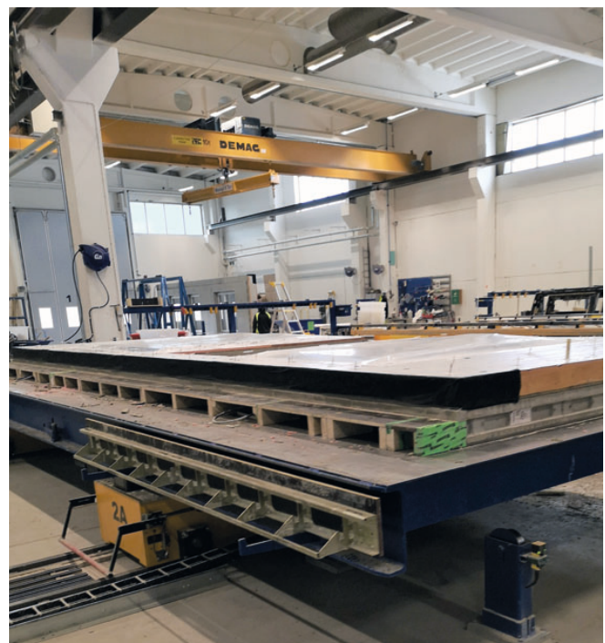
Fig. 5: Folding receptacles for shuttering transport
