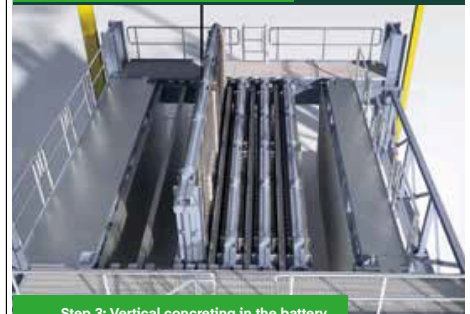
Step 3: Vertical concreting in the battery
