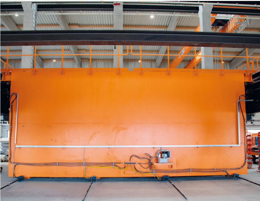
Fig. 4: Frontal view of the still unclad, movable tension wall of the butterfly battery mould; four hydraulic cylinders on the lower, longer edge of the tension wall ...
