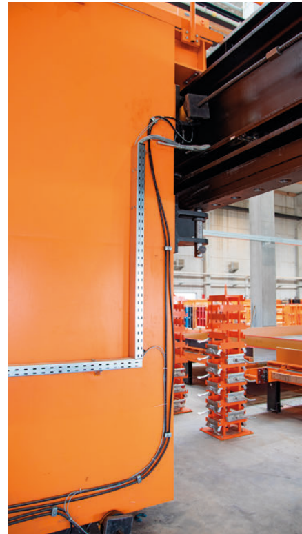
Fig. 5: ... and two hydraulic cylinders attached to the frame of the battery mould guarantee a tight closure of the casting compartments.
