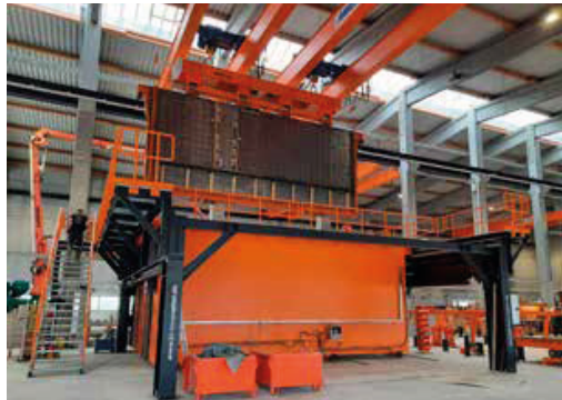
Insertion of a butterfly into the battery
