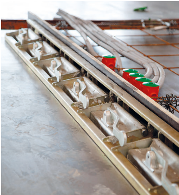
Fig. 8: For use in production at the manufacturer Beton-Fertigteile-Union, the profile of the MultiForm formwork beam was adapted and reinforced; it was also designed so that more MagFly magnets can be placed at smaller distances from each other. The shuttering can thus withstand high pressure when concreting vertically in the butterfly battery mould.
