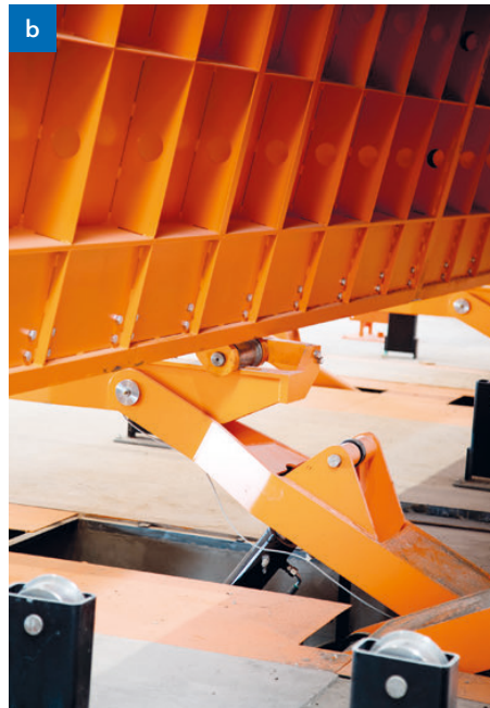
Fig. 9a+b: A lifting beam is connected to the hinge of the butterfly formwork.
