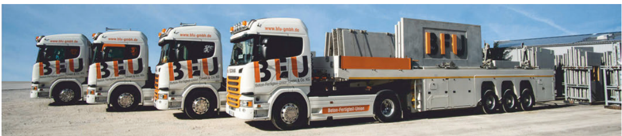
Fig. 12: Ready for transport – with BFU's own trucks and inloaders from Faymonville, the high-quality, fair-faced precast concrete elements reach the construction sites in the southern German state of Baden-Württemberg and in neighbouring Switzerland.
