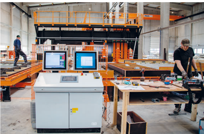
Fig. 6: The control panel for the two work stations, with a butterfly formwork each lying open (immediately to the left and right behind it) and the side view of the battery mould in the background – the battery mould has its own control panel.
