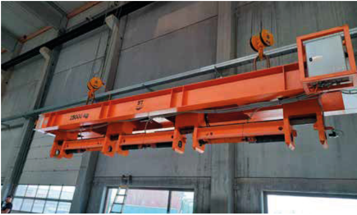
Custom lifting beam for butterflies
