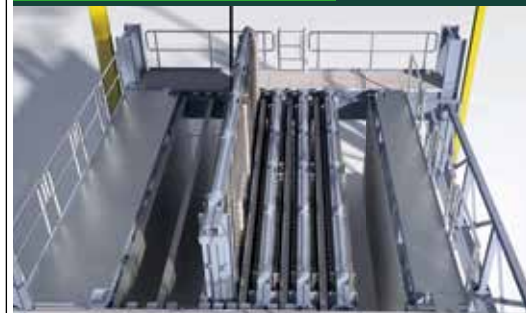
Step 3: Vertical concreting in the battery
