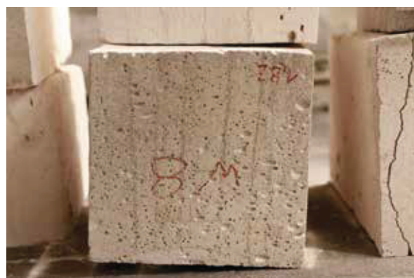
Figure 2 (right): The test cubes cut out of the completed wall were used for determining the density and the compressive strength. The test cubes and the background of the diagram on the left provide information on the surface quality of the material.
