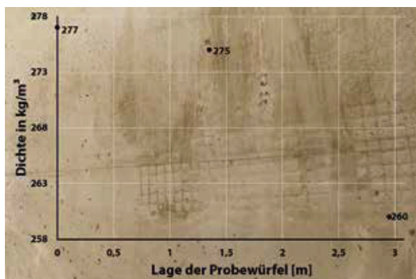
Figure 1 (left): From the foamed-concrete wall, five test cubes each were cut out for determining density. The position of the cubes corresponds to the distance from the lower edge of the cut-out cube to the lower edge of the cast foamed-concrete wall.
